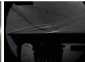
Flow studies using cone models and Schlieren flow visualization studies of the induced shock
